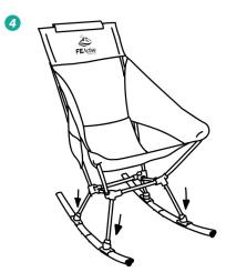
Align the four outer ridges on the rockers with the chair legs. Push them together until they snap into place.
