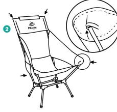
Carefully attach the 4 corners of the fabric to the corresponding poles that are pointing upwards.
