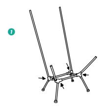
Securely attach all poles to the corresponding holes. Use the internal bungee cords and plastic inserts to bind the frame and legs together.
