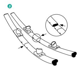
The rocker's chair legs come in two pieces. Slide the pieces into place and push the pins until they lock.
